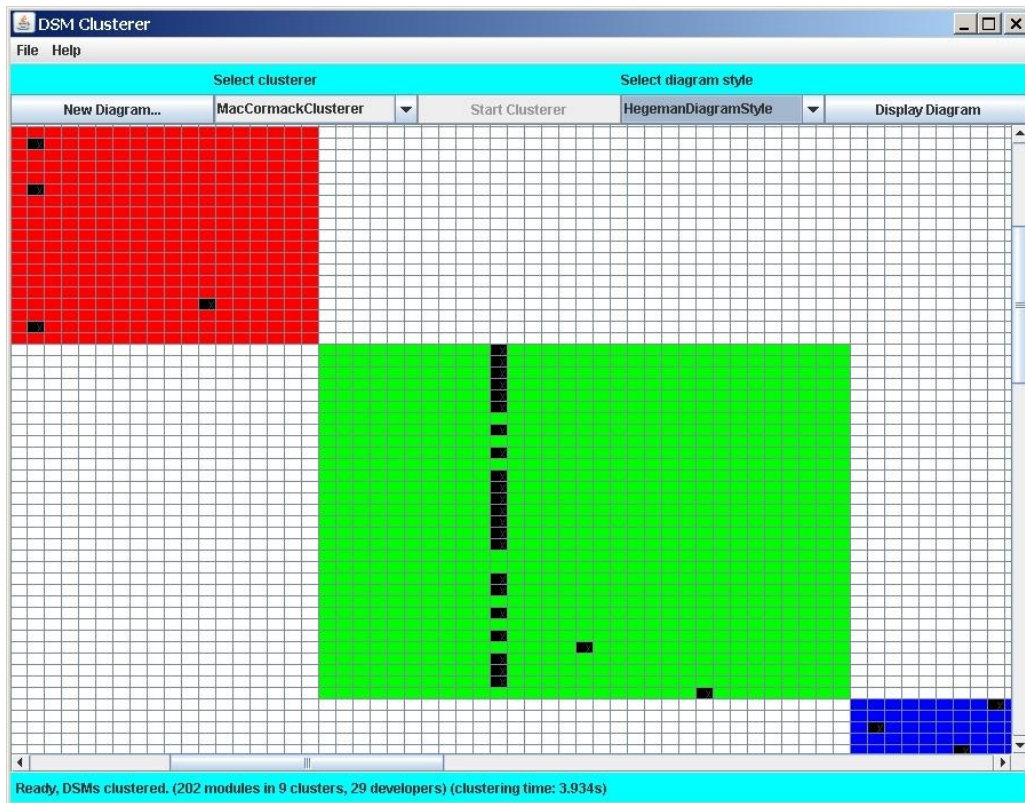
Figure 15: A clustered DSM in the DSMCluster tool
